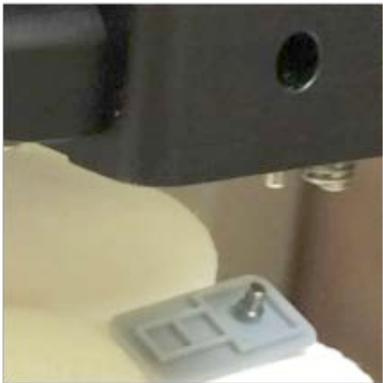
1. With appropriate hand protection in place, remove the nozzle plate using a 3 mm torque allen wrench. If the diaphragm has become stuck to the heater block, use a probe or an appropriate tool to carefully remove it.
