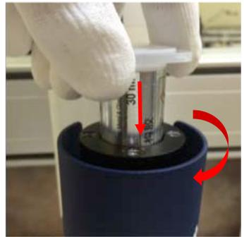
9. Replace the receiver head (top air supply) and tighten the thumbscrews.
