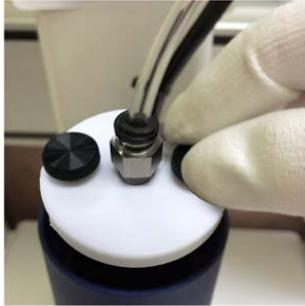
2. Lower the hot melt feed tube down into the melter so it extends out of the bottom.
