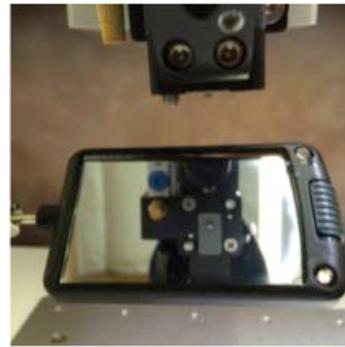
6. Align the Nozzle Plate to the alignment pins on the Heater Block. Make sure the O-ring faces up and the fluid barb faces the melter.
