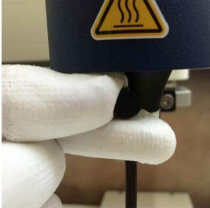
6. Loosen the receiver head thumbscrews and remove the receiver head (top air supply).
