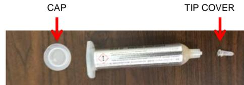
8. Use a probe to pry up the syringe of melted PUR material. Remove the syringe and feed tube. Discard the feed tube. Replace the tip cap and top cap before discarding the syringe.
